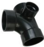
3" x 3" x 3" x 2" Right Side Inlet ABS Sanitary Tee
