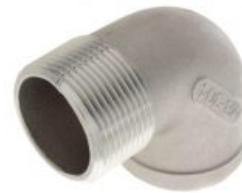
1-1/4" 316 Stainless Steel Street 90 Degree Elbow
