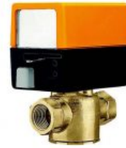
3/4" Female NPT Belimo Zone Valve, 5.0 CV
