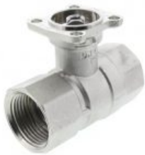
1-1/2" Belimo 2-Way, Characterized Control Valve Female NPT, 29 Cv
