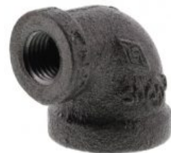
1/2" x 1/4" Black Malleable Reducing 90 Degree Elbow
