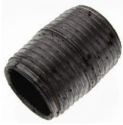
1/2" x Close (1-1/8") Black Steel Nipple (Sch 40)
