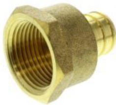
1-1/4" Female NPT x 1-1/4" PEX Brass Adapter (Lead Free)
