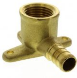
3/4" PEX x 1/2" Female NPT Brass Drop Ear Elbow (Lead Free)
