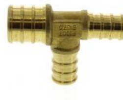
3/4" PEX x 1/2" PEX x 1/2" PEX Brass Tee (Lead Free)
