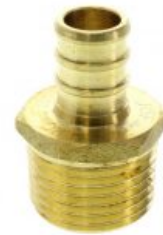
1/2" Male NPT x 1/2" PEX Brass Adapter (Lead Free)
