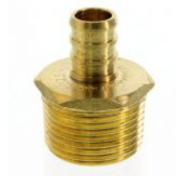
3/4" Male NPT x 1/2" PEX Brass Adapter (Lead Free)
