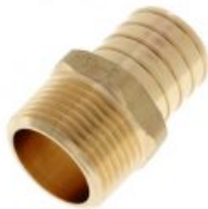
3/4" Male NPT x 1" PEX Brass Adapter (Lead Free)
