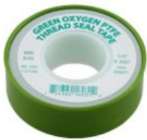
1/2" Green 260" x .004" (1.5g/cm3) High Density Oxygen T-Tape
