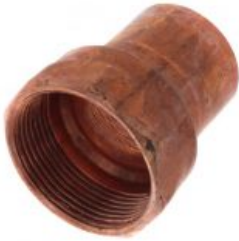
1-1/2" Male Solder (FTG) x 1-1/2" Female NPT Adapter
