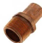
1/2" Male Solder (FTG) x 1/2" Male NPT Adapter
