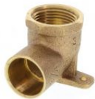
3/4" Copper x Female NPT 90 Degree Drop Ear Elbow, Lead Free
