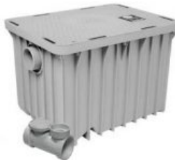
Endura20 40 lb Capacity, 20 GPM Grease Trap (2" Connection)
