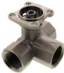
1" Belimo 3-Way, Characterized Control Valve Female NPT, 10 Cv
