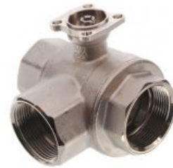
2" Belimo 3-Way, Characterized Control Valve Female NPT, 46 Cv
