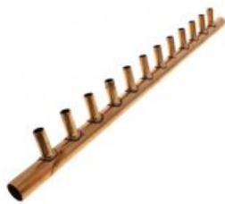
1" Male Solder (Sweat) Copper Manifold w/ 3/4" Solder, 12 Outlets
