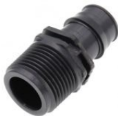
3/4" Male NPT x 3/4" F1960 Poly F1960 Expansion PEX Adapter
