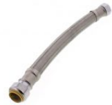
3/4" Push-Fit x 1" Female NPT Braided Water Heater Connector, 24" Length
