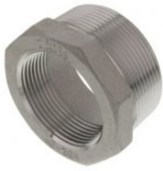
2" x 1-1/2" 316 Stainless Steel Bushing
