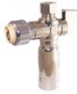
1/2" Push-Fit x 3/8" OD Comp w/ Water Hammer Arrestor, Angle Stop
