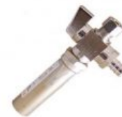
1/2" PEX Crimp x 3/8" OD Comp w/ Water Hammer Arrestor, Angle Stop
