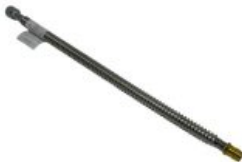
3/4" Female NPT x 3/4" F1960 Expansion PEX Stainless Corrugated Connector, 24" Long
