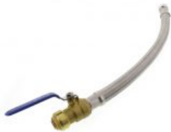
1/2" Push-Fit Ball Valve x 3/4" FIP Braided Water Heater Connector, 18" Length
