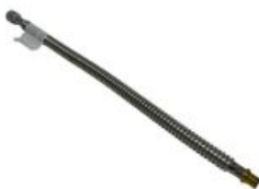
3/4" Female NPT x 3/4" F1807 Crimp PEX Stainless Corrugated Connector, 24" Long
