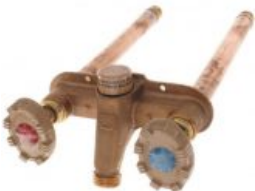
Woodford Model H22 1/2" MPT x Female Solder Anti-Siphon Hot & Cold Wall Hydrant, 12" Length
