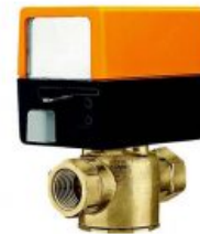
3/4" Female NPT Belimo Zone Valve, 5.0 CV
