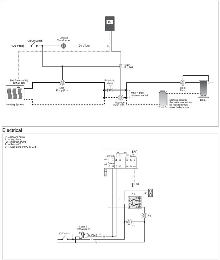
*Note:* This is only a concept drawing. Designers must determine whether this system will work in each application and must ensure compliance with code requirements. Necessary auxiliary equipment and safety devices must be added.
