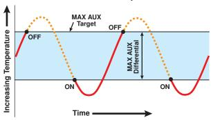
**Figure 2:** On and off points of the heat dump pump, using an auxiliary sensor in heat dump mode.
