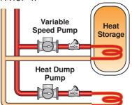
**Mode 4 Booster Pump** is for drain back applications where a booster pump is used to overcome high head upon system startup. When the  $\Delta T$  rises above the  $\Delta T$  target, the control turns on the booster pump and operates the variable speed pump at 100% output. After an adjustable time, the control turns off the booster pump and operates the variable speed pump above the minimum pump speed setting. Refer to application A157-5.
