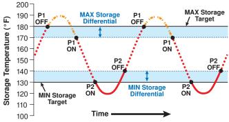
**Figure 1:** Turn on/off points for the variable speed pump (P1) and the heat supplement pump (P2) in Mode 2. The min storage target is below the max storage target. Each have a 10°F (5.5°C) differential.
