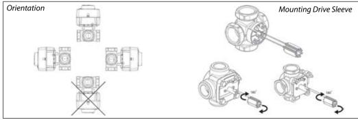
With the white drive sleeve the ARA actuator can be installed on older MG and G series of valves and also current VRG valves. The orientation of the drive sleeve determines the style of valve the actuator will mount to.
