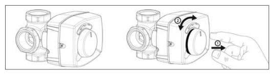
To manually operate the ARA Series actuator, slightly pull out on the large indicator knob. With it pulled out, rotate the knob to the left or right to manually operate the valve. To return the actuator to automatic operation, rotate the knob to the position prior to manual operation and push the knob into the actuator.
