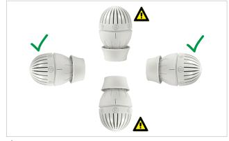
A These positions are not recommended due to the influence of the radiator temperature on the thermostatic head.
