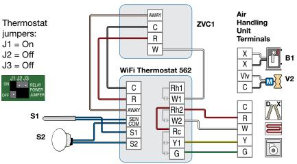
The WiFi Thermostat 562 operates a first stage baseboard/radiator and a second stage fan coil for heating, and an air conditioner for cooling.
