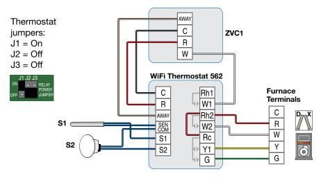
The WiFi Thermostat 562 operates a first stage radiant floor and a second stage fan coil for heating, and an air conditioner for cooling.
