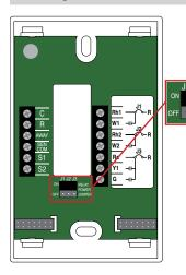
The thermostat includes three relay power jumper connectors located below the wiring hole.
