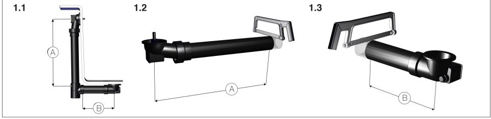
1.1: When measuring, dry fit tubing approximately 1" (2.5cm) into Tee, overflow Ell and drain Ell. Cut accordingly.
