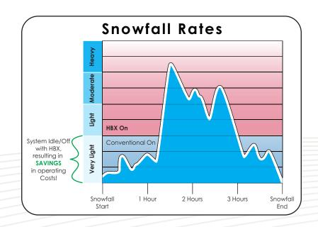
In the graph to the right, based on a "light" snowfall setting during snowfall, you can see the HBX sensor will turn on the snowmelt system much later than a conventional sensor. This results in huge savings each snow season IF your system can turn on later & turn off sooner.
