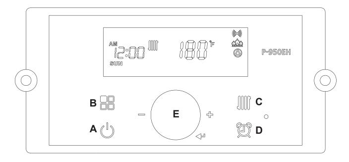
**To change CH Set point,** press the C is button. The CH Icon and current CH Set point will flash.
