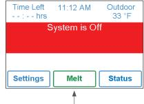
Press Melt button to start melting operation
