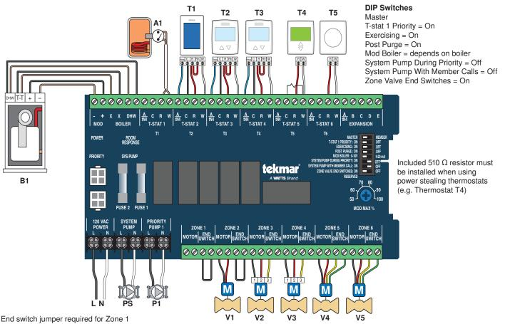
when using a pump and Zone Valve End Switch DIP = On
