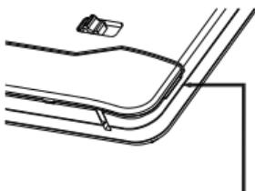
Press the lower portion of the thermostat to open the easy access battery door.
